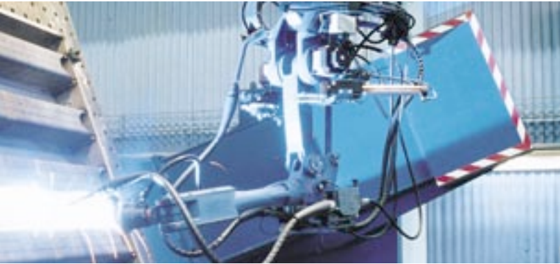
Robotic welding is used wherever possible to provide a high level of consistency and accuracy.
